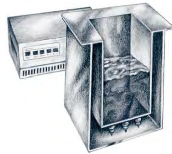
The standard batch tank is the simplest ultrasonic cleaning system available. It consists of an ultrasonic generator and a transducerized cleaning tank. The transducerized tank is constructed of stainless steel, with the transducer elements bonded to the tank bottom. The ultrasonic energy is directed upward through the tank.
